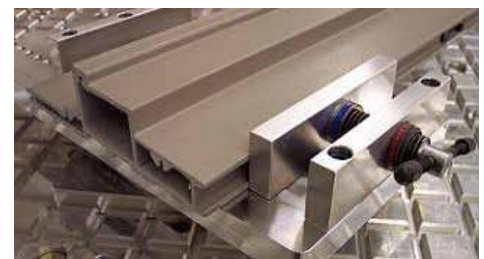
Use the NEMI Mechanical Vise top to securely clamp hard to hold materials in conjunction with our standard Slider or One Piece Vacuum Pods.
