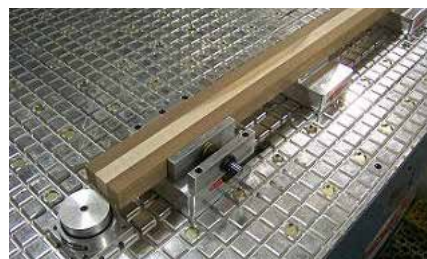
The photo above illustrates the NEMI Vise Top used in conjunction with the NEMI Modular Locator Pin and NEMI Slider Vacuum Pods.
